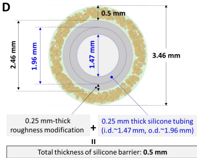
Fig. S16. Computational model development. (A) Schematics illustrating components of the control, iBEDv1, and iBEDv2 designs (left column) and iBEDv3 design (right column) including the alginate, silicone tubing, tubing lumen (air for control, iBEDv2, iBEDv3 designs, PFC for iBEDv1 design), and randomly distributed islets. (B) A high magnification image showing the randomly distributed islets in the alginate. (C) An image showing the nonuniform mesh on the alginate surface (left) and on individual simulated islets (right). (D) An annotated schematic showing the dimensions for each design.
