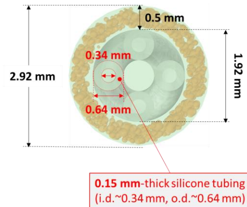
Fig. S16. Computational model development. (A) Schematics illustrating components of the control, iBEDv1, and iBEDv2 designs (left column) and iBEDv3 design (right column) including the alginate, silicone tubing, tubing lumen (air for control, iBEDv2, iBEDv3 designs, PFC for iBEDv1 design), and randomly distributed islets. (B) A high magnification image showing the randomly distributed islets in the alginate. (C) An image showing the nonuniform mesh on the alginate surface (left) and on individual simulated islets (right). (D) An annotated schematic showing the dimensions for each design.
