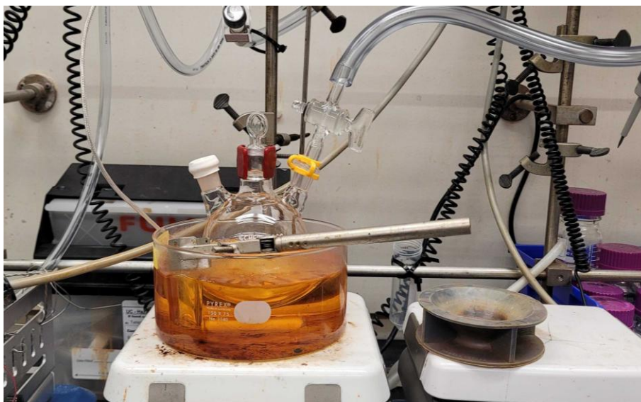
Figure 2.1.1: Experimental setup for PbS-OA NC synthesis by hot injection of substituted thiourea.
