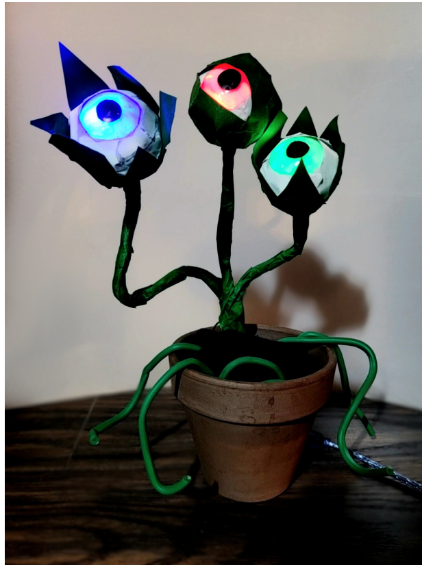
(b) A prototype of the artistic condition. Participants experience their data in a physical format through mappings of the same data to different aspects of the plant (movement, aesthetic, audio). Muscle wire is the primary actuator, and LEDs and speakers provide additional sensory output.
