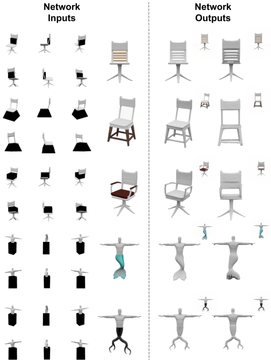
Figure B.2: Additional Qualitative Examples: Additional qualitative examples editing a chair and a full human. The left section shows the masked views and the edited conditional image. The right section shows the mesh extracted from the network output with the volumetric renders of the SDF inset.
