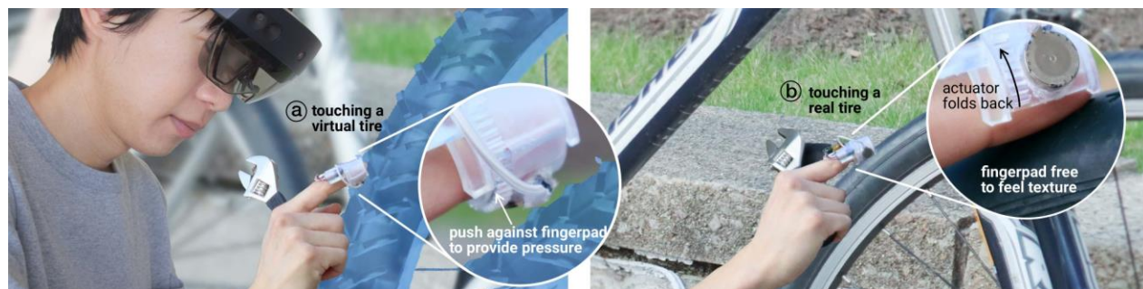
Figure 15. We engineered a foldable haptic device worn on the user’s fingernail that renders touch in mixed reality (MR) without preventing users from also touching real objects.
