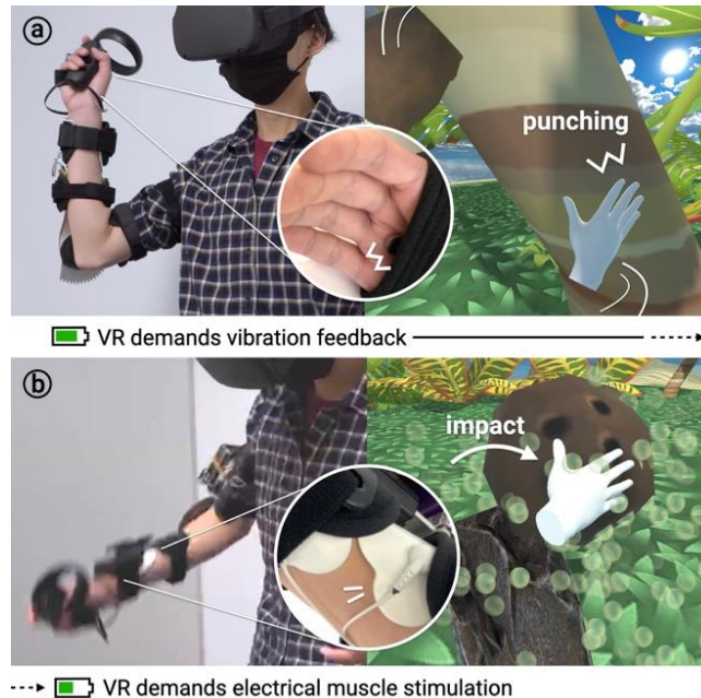
Figure 42: As the user interact with the virtual content, they feel vibrations and electrical muscle stimulation on their hand and the energy required for these haptic sensations were, unknowingly, just harvested by the user as they swam to the island.
