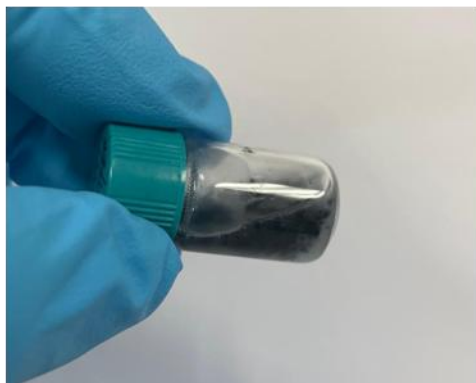
Figure S13: Optical images of bicontinuous system (BC-MP) showing thermoreversibility (inversion test)
