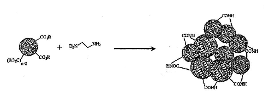
FIG. 2 Formation of a random network of Frechét-type dendrimers covalently linked with diamine compounds.
