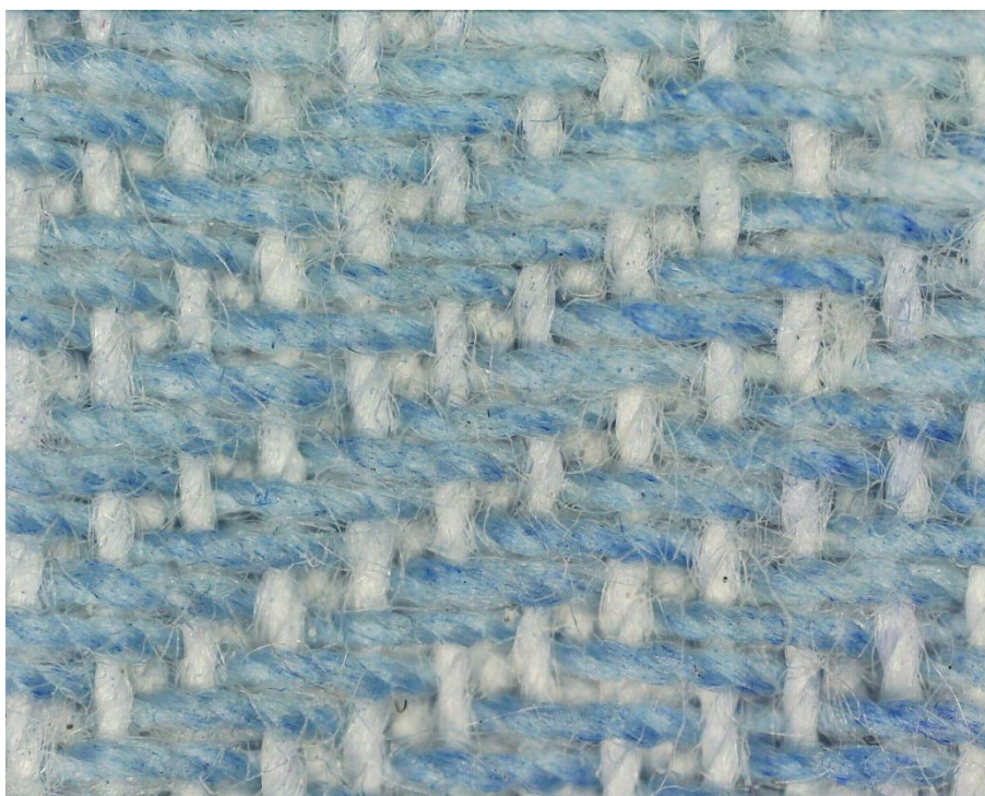
Figure S2. An optical photo of a weft-double-weave fabric.
