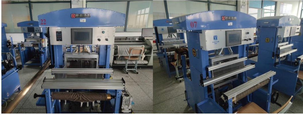
Figure S1. SGA598 semi-automatic loom for continuous UWTM weaving.
