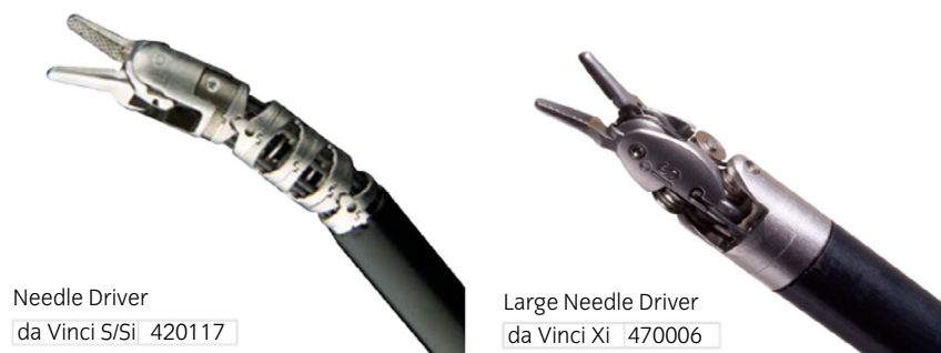
FIGURE 1 Da Vinci S/Sl 5-mm instrument with vertebral wrist (Left); Da Vinci S/Sl 8-mm instrument with articulated cardan-joint wrist (Right).
