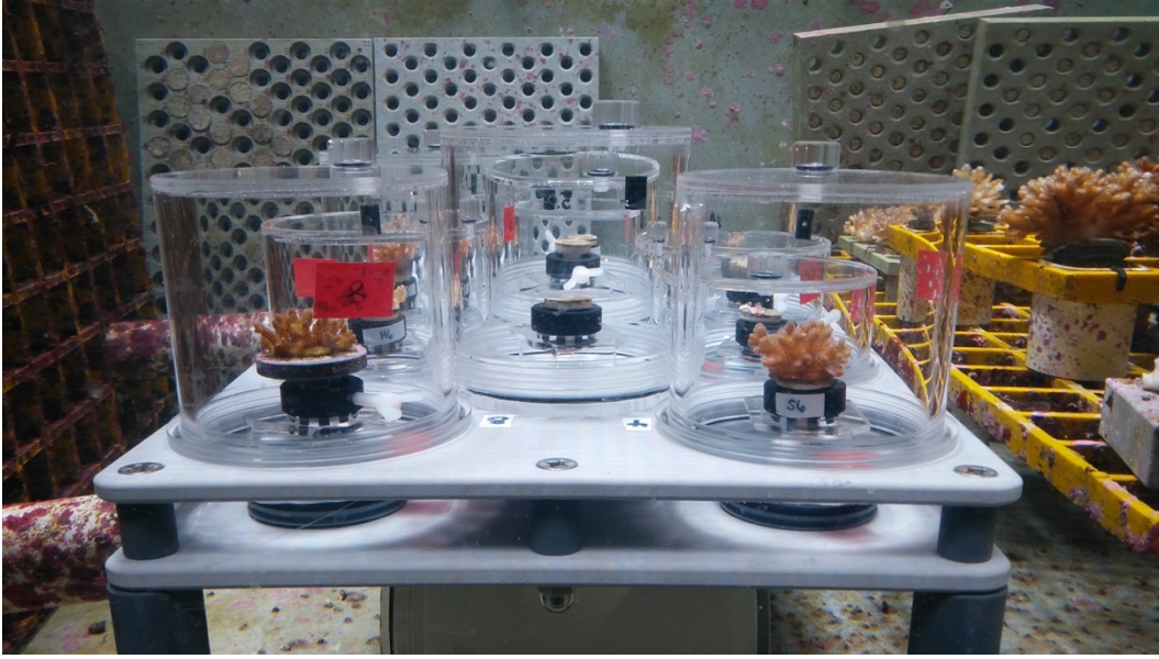
Figure 27. These P. Acutae corals from the trans-gen experiment are undergoing a periodic health check in a bespoke instrument designed by the SeaSim team to keep experimental subjects in aquaria within the aquaria for short periods of time to then test the water for changes in chemical concentrations for relevant biological functions, such as oxygen, carbon dioxide, and nitrogen for breathing. An indication that “health” goes well beyond coloration. (Source: Damien Bright)
