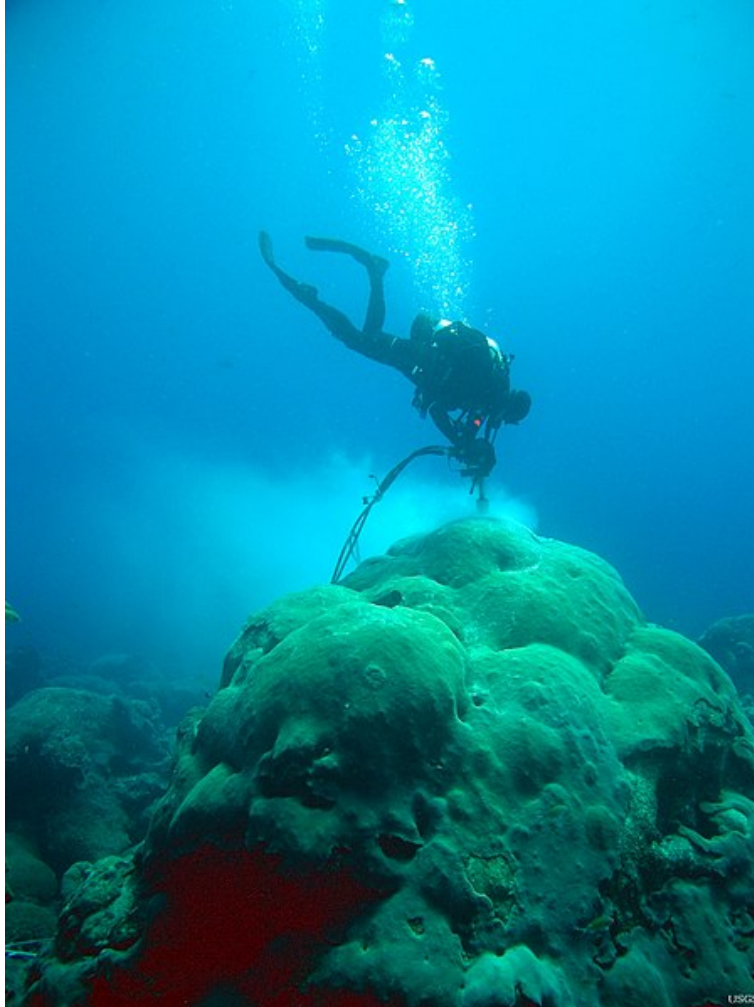
Figure 7. Christopher Reich, a United States Geological Survey diver, extracts a coral core off the coast of Florida for paleoclimatic analysis. (Source: Don Hickey, USGS, CC 1.0)
