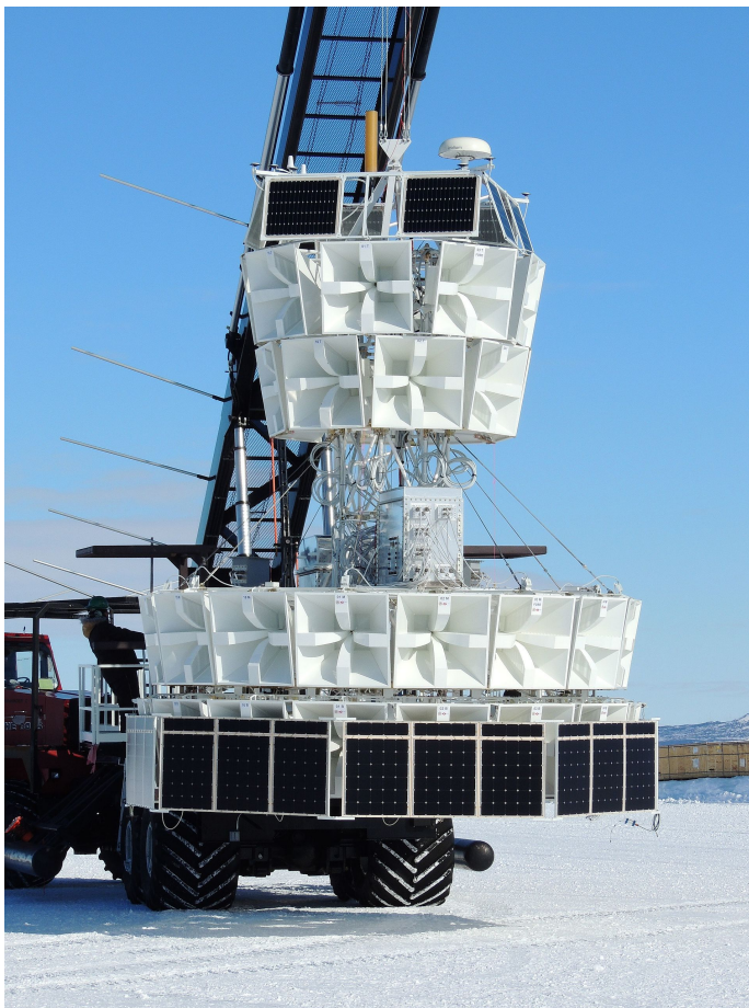
Figure 1.14: Picture of the ANITA-4 payload prior to launch near to McMurdo Station. For scale, each of the horn antennas are 0.8 m across. The solar panels on the bottom drop down after taking flight to expose another ring of antennas. Figure from [95], available under Creative Commons licensing.
