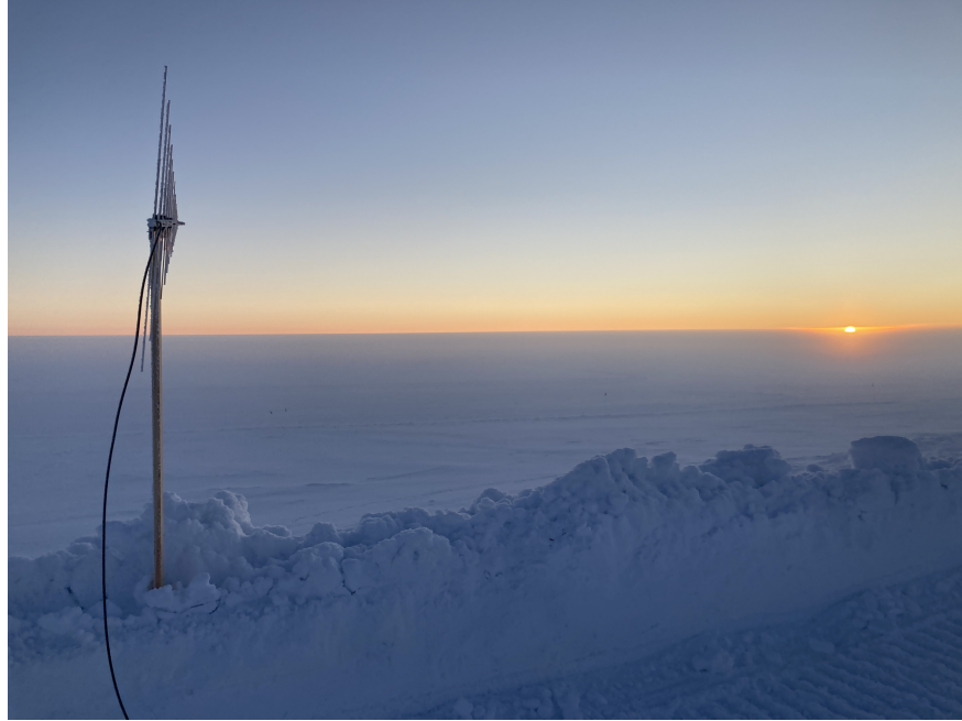
Figure 2.35: Photo of ‘berm-top’ pulsing, showing an LPDA broadcasting to the three stations deployed in Summer 2021.
