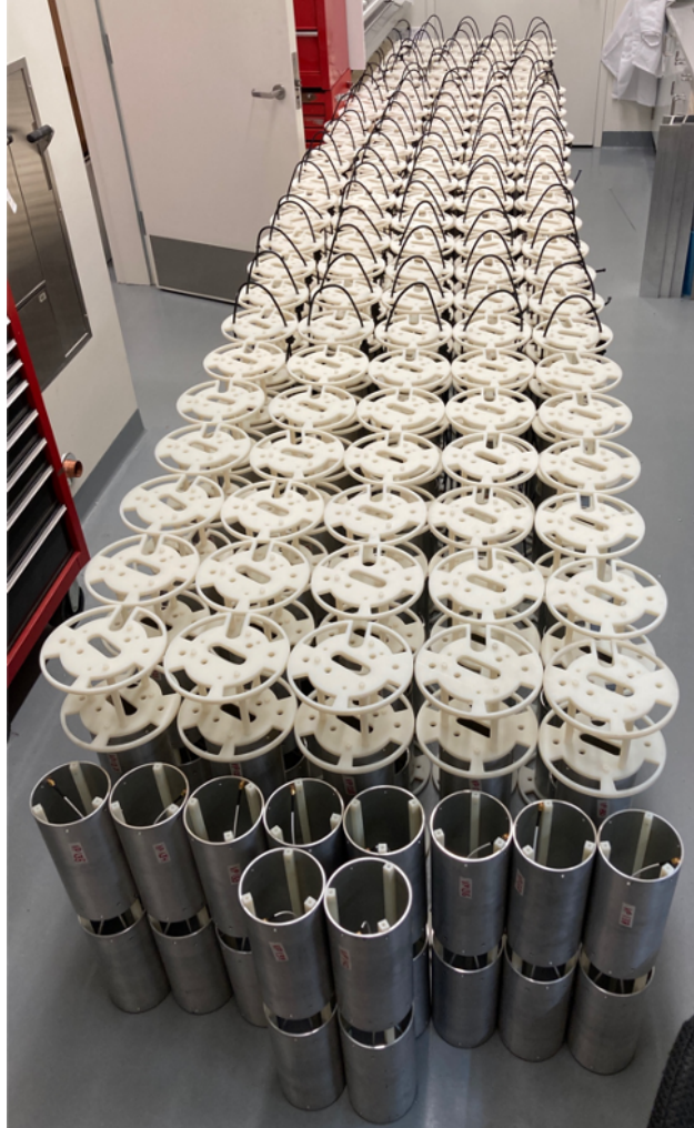
Figure 2.22: Picture of the 145 VPol V2 antennas assembled before shipment to Summit Station.
