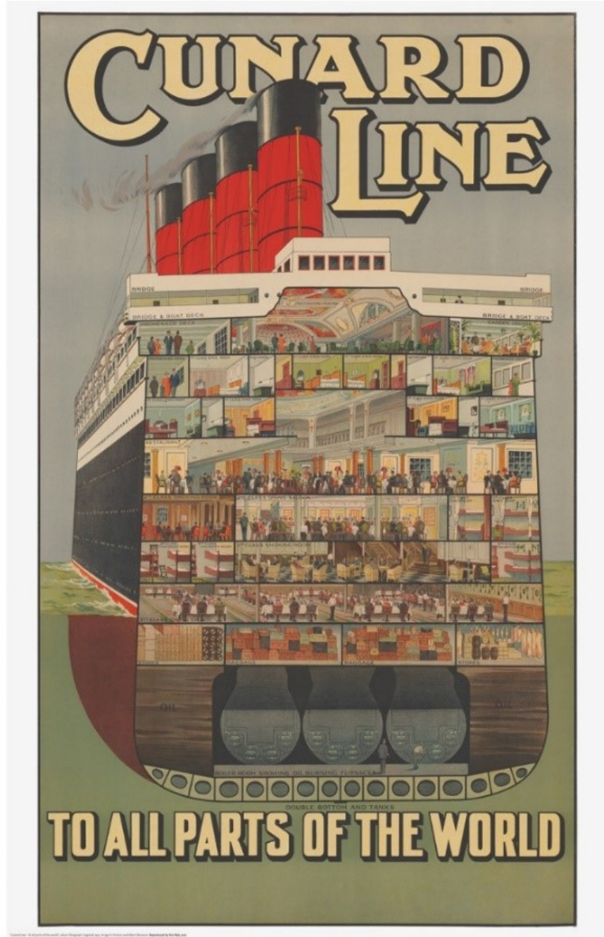
Figure 16. Cross-section image of the Cunard steamship “Aquitania” commissioned by Cunard Lines. Note that the ship has made the transition from coal to oil. Ulrich Guttersohn, “Cunard – To all parts of the world.” Color lithograph printed by Thomas Forman & Sons Ltd. in Nottingham, c. 1914. Victoria and Albert Museum, London (E. 1829-2004).
