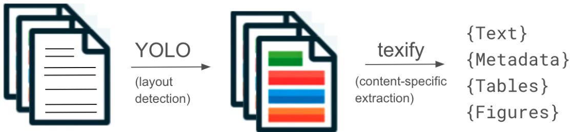
Figure 3.2: Parsing workflow for scientific PDFs. Oreo allows content-aware extraction of information from large-scale PDF collections by combining a YOLO-based layout detector with the Texify Vision Transformer for content-specific extraction. The two-stage design produces a 4.5\times speedup over Nougat [18] and a 94.6\times improvement in FLOP utilization, while supporting 20 categories of document elements.
