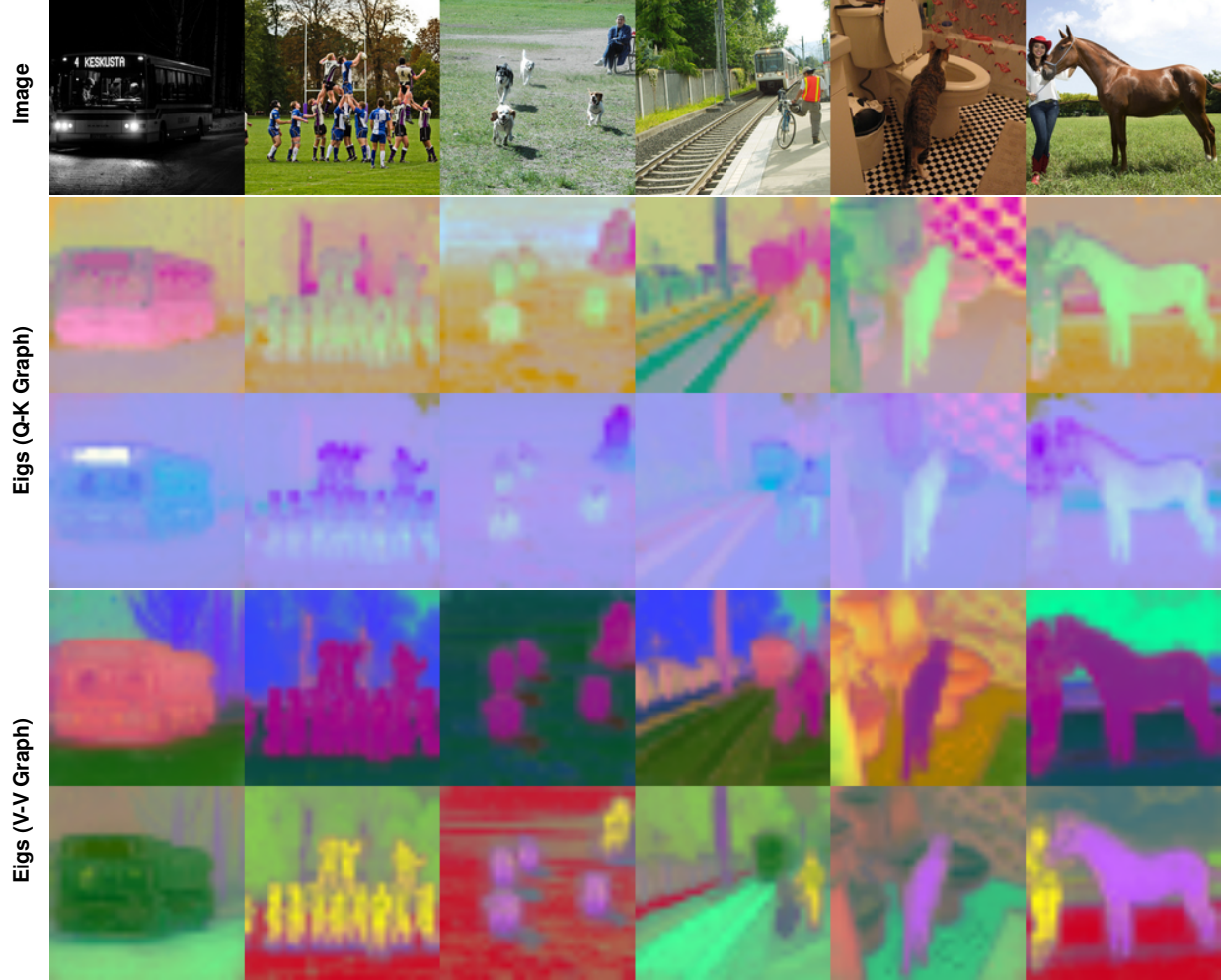
Figure 4.5: Extracted eigenvectors on COCO for both graph choices. We visualize selected components of \mathbf{X}_{\text{ortho}} , sorted by decreasing eigenvalue. Three eigenvectors at a time are rendered as RGB images. In the Q-K case, the first set of eigenvectors describes general scene spatial layout in terms of ground, subject, background, and sky. The second finds top-to-bottom part separation within objects. In the V-V case, the first set of eigenvectors partitions the image into coarse semantics like trees, ground, and sky, while the second set recognizes finer-grained categories and groups individual objects like people, animals, and vehicles.
