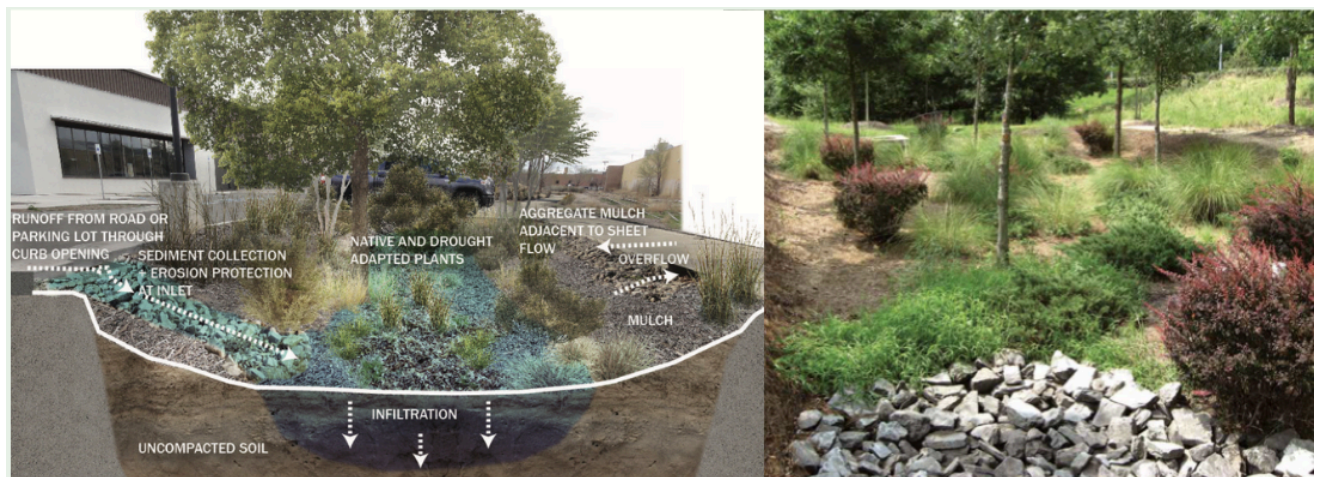
Figure 5. Structural diagram and image of bioretention cells designed for infiltration (i.e infiltration basins). Courtesy of San Antonio River Authority, Bexar Regional Watershed Management
