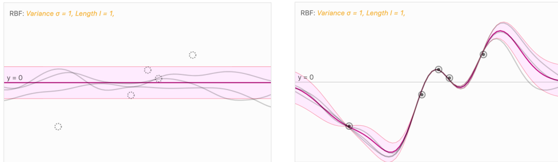
(Left) The prior distribution of a Gaussian process with a RBF kernel. (Right) The situation after datapoints have been observed. The mean prediction is shown as the pink line and three samples are shown as gray lines. In both plots the shaded region denotes twice the standard deviation at each input value x .
