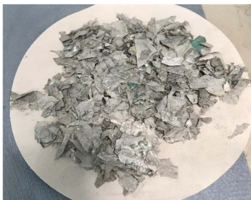
Figure 25. Flaked (light fraction) plastic (from figure 24) following enhanced laboratory scale chemical cleaning processes.
