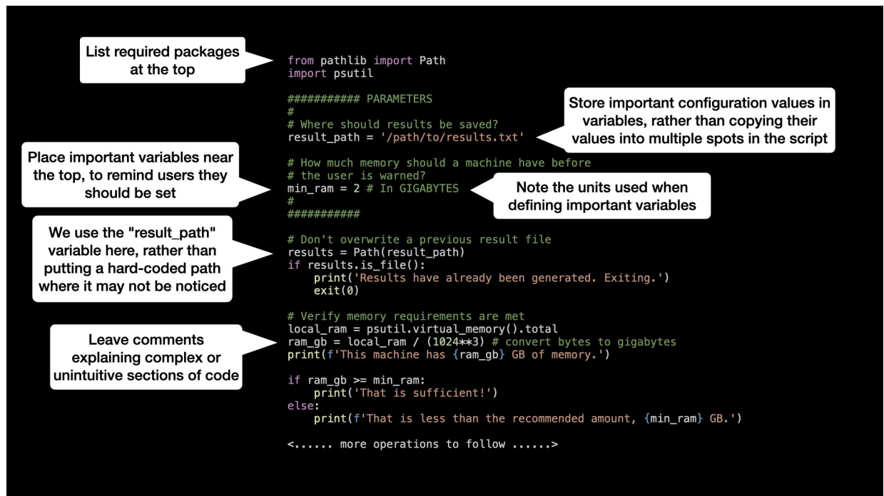
Fig 1. Example code for a reproducible project. The first lines of a longer analysis script written in Python 3 with examples of practices that make the code easier for other users to understand.
