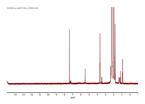
Figure S7. <sup>1</sup>H NMR of 20  $H_2O$  + 20 AgOTf in CD<sub>3</sub>CN.
