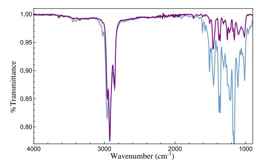
Figure S21. Full IR of crude **2** as a thin film (blue) and IR of **2** made in the presence of 2,6-lutidine as a thin film (purple).
