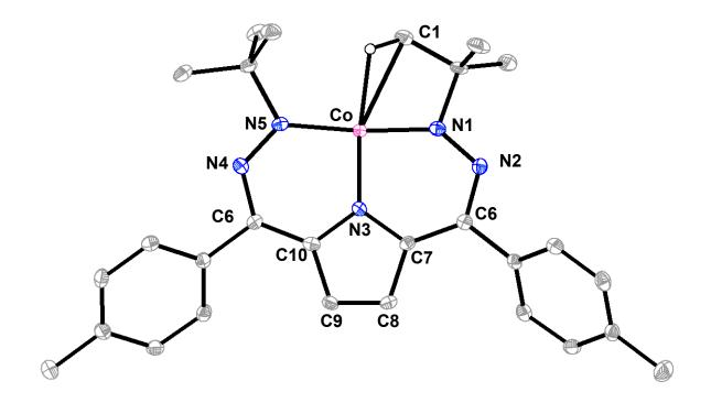
Figure S37. SXRD of **2**. Co (pink), N (blue), C (gray), H(white). Most C-H H-atoms omitted. Selected bond lengths (Å): Co-N1/N5: 1.796(2), 1.847(2); Co-N3: 1.821(2); N1-N2/N4-N5: 1.323(2), 1.318(2); Co-C-H: 1.770(2); N2-C5/N4-C10: 1.343(3), 1.336(3); C5-C6/C9-C10: 1.403(3), 1.402(3); C6-C7/C8-C9: 1.436(3), 1.433(3); C7-C8: 1.353(3). Selected bond angles (°): N1-M-N5: 172.33(8); N3-M-(C-H): 162.15(8).
