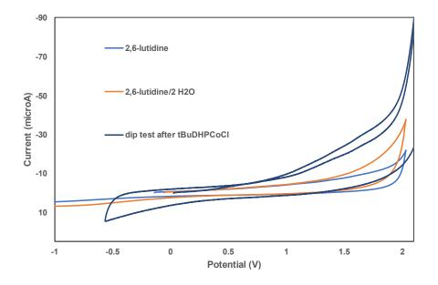
Figure S26. Cyclic Voltammogram of 0.16 M 2,6-lutidine, 0.32 M  $H_2O$  and 0.16 M 2,6-lutidine, and a dip test of a used electrode in 0.32 M  $H_2O$  and 0.16 M 2,6-lutidine in 0.1 M  $NBu_4PF_6$  acetonitrile.
