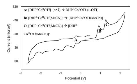
Figure S25. Cyclic Voltammogram of 1 mM of 1-OTf in 0.1 M NBu<sub>4</sub>PF<sub>6</sub> acetonitrile.
