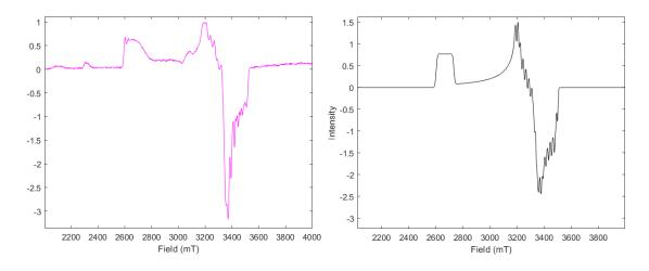
Figure S22. Small Window perpendicular-mode EPR spectrum (left) and simulated spectrum (right) of a 15 mM solution of **1** in toluene at 15 K. Conditions: MW frequency, 9.631 GHz; MW power, 2.0 mW.
