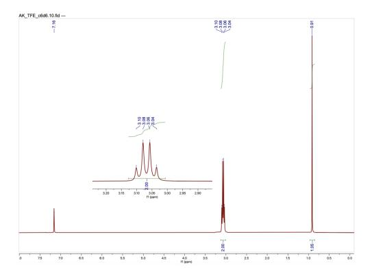
Figure S5. <sup>1</sup>H NMR of 2,2,2-Trifluoroethanol (TFE) in C<sub>6</sub>D<sub>6</sub>.
