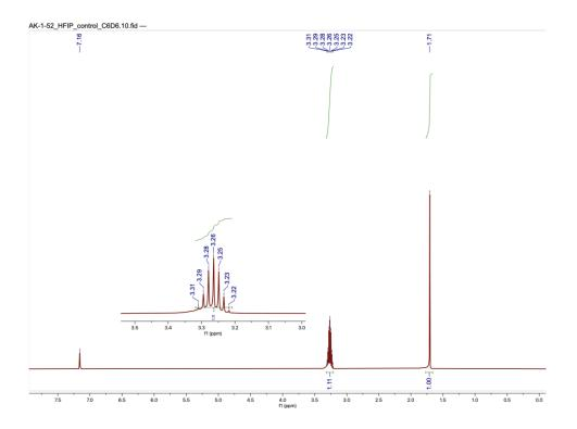
Figure S3. 1H NMR of (CF<sub>3</sub>)<sub>2</sub>CHOH (HFIP) in  $C_6D_6$ .
