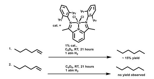
Figure S89. Controls (1.) with alternative cobalt catalyst<sup>16</sup> and (2.) with no cobalt-containing species. Some yield is observed from the alternative catalyst, but it is significantly less than that observed with 2, and no quantifiable yield was observed in the absence of cobalt catalyst.
