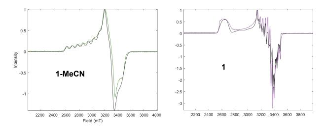
**Figure 3.** Complex **1-MeCN** (left) at 15.9 K and Complex **1** (right) at 15.9 K. **1-MeCN**: g = 2.0585, 2.0788, 2.1315; Co-A = +15.9328, +9.9042, 57.2366 MHz, N-A = +58.4688, +19.2988, +30.0000 MHz. **1**: g = 2.0598, 2.0766, 2.1739; Co-A = +10.8252, +22.5562, +5.6313 MHz; N-A = +31.5100, -8.0770, +30.9039 MHz. microwave frequency 9.6304 GHz, microwave power 0.2 mW.
