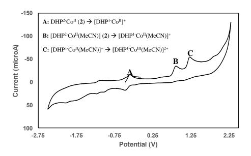
Figure S23. Cyclic Voltammogram of 1 mM of 2 in 0.1 M NBu<sub>4</sub>PF<sub>6</sub> acetonitrile.
