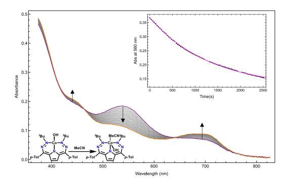
Figure S13. First intermediate formation in the reaction of **1-OH** (0.094 mM) with MeCN at 2  $^{\circ}$ C in diethyl ether with inset of the trace at 560 nm with the first-order fit of that data in magenta. Equation 1. Derivation of fit shown above in Figure S13.<sup>1</sup>
