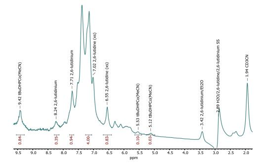
Figure S3. <sup>1</sup>H NMR in CD<sub>3</sub>CN of reaction between (<sup>*t*Bu,Tol</sup>DHP)CoCl (**1**) in Et<sub>2</sub>O, H<sub>2</sub>O, 2,6lutidine, and NaI. Products observable are (<sup>*t*Bu,Tol</sup>DHP)Co(MeCN) (**2-MeCN**), 2,6-lutidinium chloride, and residual 2,6-lutidine.
