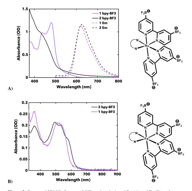
**Figure 3.** Compared UV-Vis Spectra of differently substituted Ru (A) and Fe (B) analogs. Excitingly, the Ru spectrum changes shape dramatically and there is a shoulder at 600 nm in the Fe spectra that suggests potentially we are observing the triplet iron complex.
