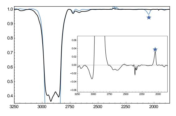
Figure S14. Zoomed IR with difference spectrum inset of **3** (black) and **3-D**<sub>2</sub> (blue) in nujol. Star indicates the N–D stretch.
