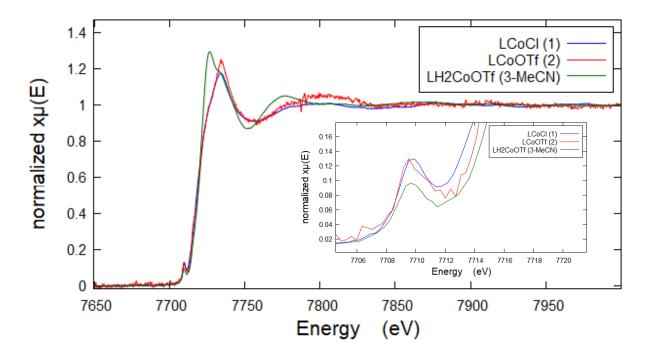
Figure S30. X-ray absorption spectra of **1** (blue), **2** (red) and **3-MeCN** (green) with pre-edge features at 7709.7, 7709.3, and 7709.3 eV respectively. These were all collected as frozen solutions at 183 K, with **1** and **2** in toluene and **3-MeCN** in a 1:4 MeCN:toluene mixture.
