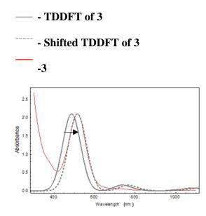
Figure S87. TDDFT of 3. Note that TD-DFT typically underestimates the energies of transitions and a shift to match experimental data of 50-75 nm is common in the related Ni- and Fe-DHP complexes.
