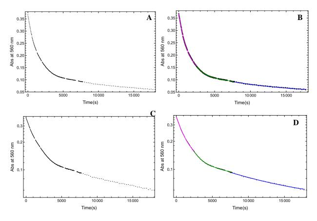
Figure S12. From left to right and top to bottom, A- Trace of the Reaction at 560 nm of **1-OH** (0.094 mM) with MeCN at 2 °C in diethyl ether, B- Fitted Trace of the Reaction at 560 nm of **1-OH** with MeCN at at 2 °C in diethyl ether, C- Log plot of 1 and D-Log plot of **2**.
