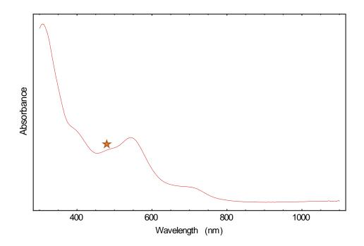
Figure S4. UV-vis of **1** from a 0.13 mM solution in toluene at room temperature. Orange marker indicates presence of putative thermal decomposition product (assigned as **2**)
