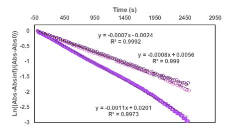
Figure S14. Linear fits for k in the first order fits of the data shown above (as well as a check for reproducibility in the reaction of **1-OH** at 0.094 mM, 0.043 mM, and 0.078 mM) with MeCN at 2  $^{\circ}$ C in diethyl ether. k<sub>obs</sub> = 0.0009(2).
