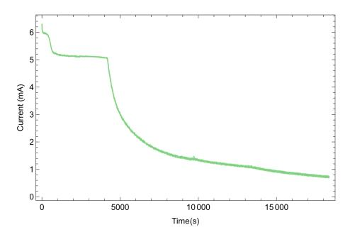
Figure S32. Bulk electrolysis at 1400 mV of 1 mM **1**, 320\*2 equiv. H<sub>2</sub>O (320 in each divided cell compartment) and 160 equiv. 2,6-lutidine in 0.1 M NBu<sub>4</sub>PF<sub>6</sub> acetonitrile.
