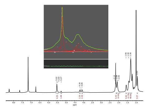
Figure S101. <sup>1</sup>H NMR of 2.5 mol%: 1 isomerization of trielaidin under standard photochemical conditions in  $C_6D_6$  with 1 µL mesitylene internal standard. Integration of various products done directly via curve-fitting in Fityk (inset included).
