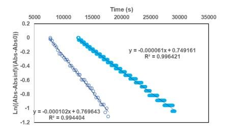
Figure S18. Linear fits in the second order fits of the data shown above (as well as check for reproducibility in the reaction of 1-OH at 0.094 mM, 0.043 mM, and 0.078 mM) with MeCN at 2  $^{\circ}$ C in diethyl ether. K<sub>obs</sub> = 0.00008(2).
