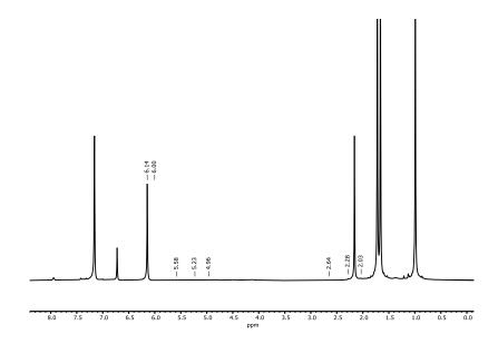
Figure S100. <sup>1</sup>H NMR of 2.5 mol%: 1 isomerization of 2,5-dimethylhexa-2,4-diene under standard photochemical conditions in  $C_6D_6$  with 1 µL mesitylene internal standard. Integration of various products done directly.
