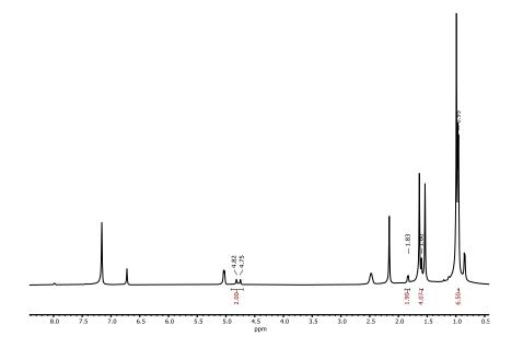
Figure S97. <sup>1</sup>H NMR of 2.5 mol%: 1 isomerization of 2,4-dimethylpent-2-ene under standard photochemical conditions in  $C_6D_6$  with 1 µL mesitylene internal standard. Integration of various products done directly.
