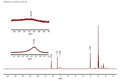
Figure S5. <sup>1</sup>H NMR of (<sup>*t*Bu,Tol</sup>DHP)CoOTf (**1-OTf**) in CD<sub>3</sub>CN.
