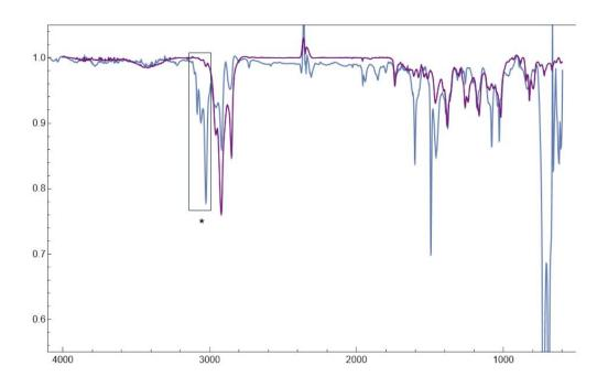
Figure S15. IR comparing IR of **1** (purple) as a thin film to IR of [<sup>*t*Bu, Tol</sup>DHP]CoOH (blue) as a thin film.
