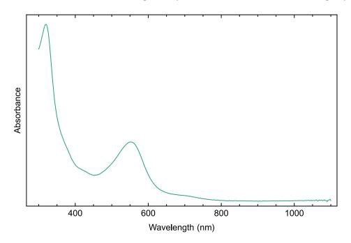
Figure S8. UV-vis of **2** from a 0.106 mM solution in diethyl ether at room temperature.
