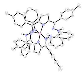
**Figure 11.** Cobalt homoleptic complex with phenyl analog of ligand—from an attempt to metallate! [<sup>Ph,Tol</sup>DHP-H<sub>2</sub>]Co[<sup>Ph,Tol</sup>DHP-H], Co (pink), N (blue), C (gray). C-H-atoms were omitted for clarity.
