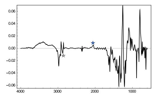
Figure S17. IR difference spectrum of **3** (black) and **3-D**<sub>2</sub> (blue) as a thin film on KBr. Blue star indicates the N–D stretch. Gray star indicates the proposed position of the N–H stretch.
