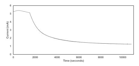
Figure S34. Bulk electrolysis at 1400 mV of 320\*2 equiv. H<sub>2</sub>O (320 in each divided cell compartment), CoCl<sub>2</sub> and 160 equiv. 2,6-lutidine in 0.1 M NBu<sub>4</sub>PF<sub>6</sub> acetonitrile.
