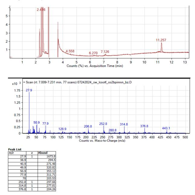
Figure S103. GCMS of dried post-thermal isomerization reaction of 1-hexene with HBPin. With the olefins and other volatile residues removed, all that is observable is residual solvent peaks from the instrument below 3 minutes, a peak at 7.126 with masses corresponding to a hydroborated ligand, and a peak at 11.257 consistent with free ligand.
