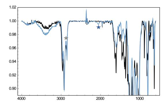
Figure S16. IR of **3** (black) and **3-D**<sub>2</sub> (blue) as a thin film on KBr. Blue star indicates the N–D stretch. Gray star indicates the proposed position of the N–H stretch.
