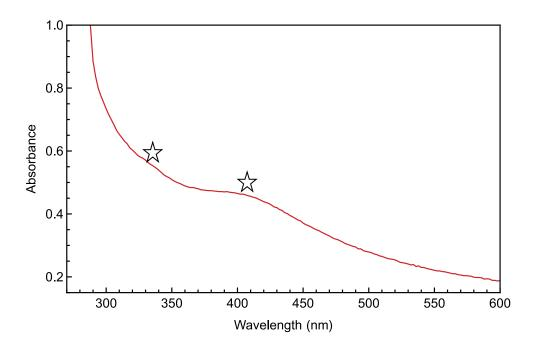
Figure S11. UV-vis of  $I_3^-$  generated from  $H_2O_2$  product and NaI from a solution in water at room temperature.
