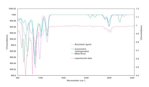
Figure S20. IR of **2-BPin** as a thin film (pink) with comparison DFT-calculated IRs for hydroborated ligand (purple), asymmetric hydrogenation of the ligand (blue), and a metal boryl species (green) shown.
