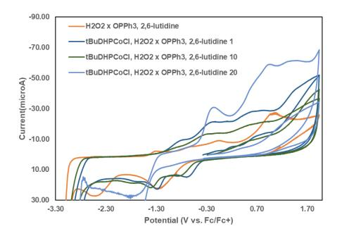
Figure S36. Cyclic Voltammograms of 1 mM **1** in the presence of H<sub>2</sub>O<sub>2</sub>•2-OPPh<sub>3</sub> and 160 equiv. 2,6-lutidine in 0.1 M NBu<sub>4</sub>PF<sub>6</sub> acetonitrile.
