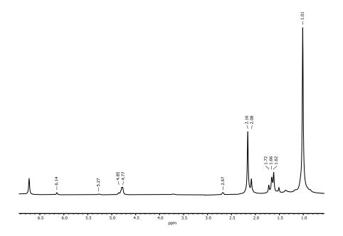
Figure S99. <sup>1</sup>H NMR of 2.5 mol%: 1 isomerization of 2,5-dimethylhexa-1,5-diene under standard thermal conditions in  $C_6D_6$  with 1 µL mesitylene internal standard. Integration of various products done directly.
