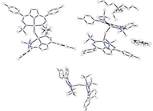
**Figure 7.** Oxo or Hydroxide bridged dimer—formed from potassium oxide cobalt complex attempt for a cyclic voltammogram in NBu<sub>4</sub>PF<sub>6</sub> electrolyte. [<sup>*t*Bu,Tol</sup>DHP]CoO(H?)Co[<sup>*t*Bu,Tol</sup>DHP](NBu<sub>4</sub>), Co (pink), N (blue), C (gray), O (red). C-H-atoms were omitted for clarity. 355
