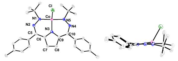
Figure S32. SXRD of **1**. Co (pink), N (blue), C (gray), Cl (green), H-atoms omitted. Selected bond lengths (Å): Co-N1/N5: 1.883(4), 1.891(5); Co-N3: 1.861(4); N1-N2/N4-N5: 1.303(6), 1.288(6); Co-Cl: 2.198(2); N2-C5/N4-C10: 1.343(7), 1.338(7); C5-C6/C9-C10: 1.388(8), 1.383(8); C6-C7/C8-C9: 1.434(8), 1.433(8); C7-C8: 1.351(8). Selected bond angles (°): N1-M-N5: 164.7(2); N3-M-Cl: 129.1(2). Table S2. SXRD of 1.
