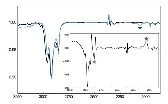
Figure S18. Zoomed IR with difference spectrum inset of **3** (black) and **3-D**<sub>2</sub> (blue) as a thin film on KBr. Blue star indicates the N–D stretch. Gray star indicates the proposed position of the N–H stretch.
