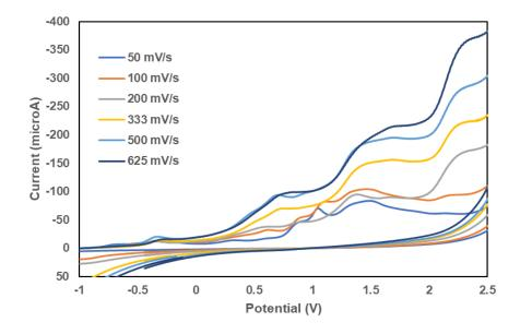
Figure S30. Cyclic Voltammograms of 1 mM  $\mathbf{1}$ , 320 equiv. H<sub>2</sub>O and 160 equiv. 2,6-lutidine at varied scan rates in 0.1 M NBu<sub>4</sub>PF<sub>6</sub> acetonitrile.
