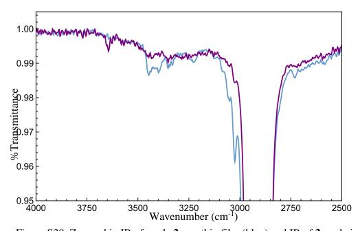
Figure S20. Zoomed in IR of crude **2** as a thin film (blue) and IR of **2** made in the presence of 2,6-lutidine as a thin film (purple). This data clearly shows additional peaks in the N-H region that are suppressed and replaced with a singular N-H peak in the presence of a base (2,6-lutidine, the base, becomes 2,6-lutidinium chloride)
