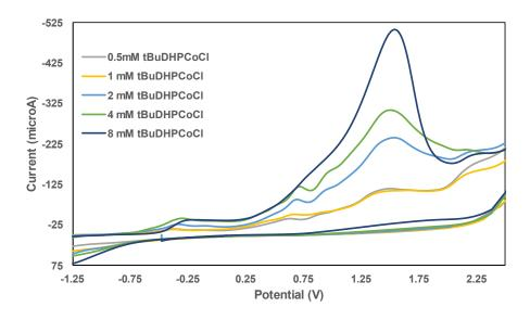
Figure S31. Cyclic Voltammograms of  $0.32 \text{ M H}_2\text{O}$  and 0.16 M 2,6-lutidine in the presence of varied amounts of **1** in 0.1 M NBu<sub>4</sub>PF<sub>6</sub> acetonitrile.
