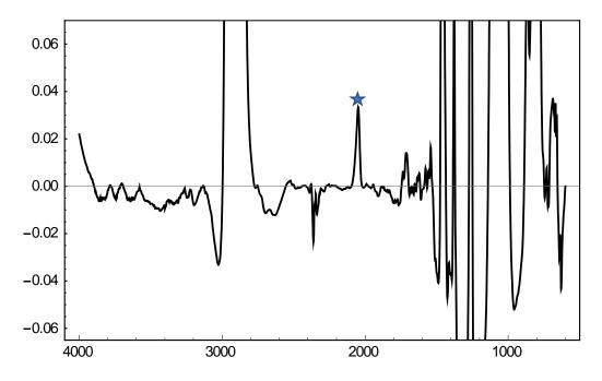
Figure S13. IR difference spectrum of **3** (black) and **3-D**<sub>2</sub> (blue) in nujol. Star indicates the N–D stretch.
