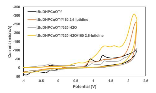
Figure S28. Cyclic Voltammograms of 1 mM **1-OTf**,  $H_2O$  and 2,6-lutidine in 0.1 M NBu<sub>4</sub>PF<sub>6</sub> in acetonitrile.
