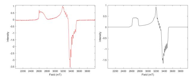
Figure S27. Small Window perpendicular-mode EPR spectrum and simulated spectrum overlay of a 15 mM solution of **3** in toluene at 20 K with 9.0% 2 impurity included. Conditions: MW frequency, 9.631 GHz; MW power, 2.0 mW.
