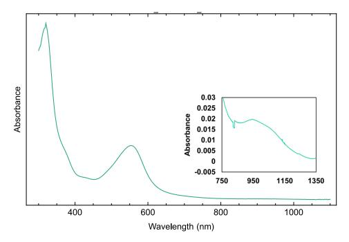
Figure S10. UV-vis of **1-OH** from a 0.153 mM solution in diethyl ether at room temperature.
