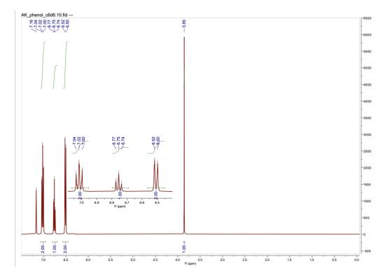
Figure S6. <sup>1</sup>H NMR of Phenol in C<sub>6</sub>D<sub>6</sub>.
