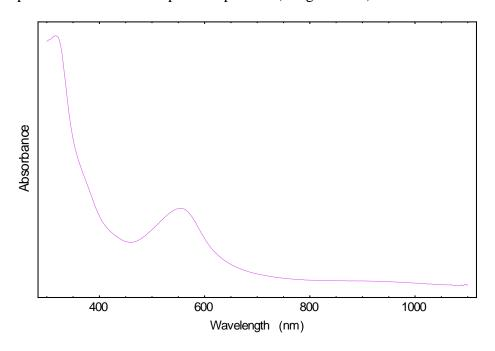
Figure S6. UV-vis of 3 from a 0.21 mM solution in toluene at room temperature
