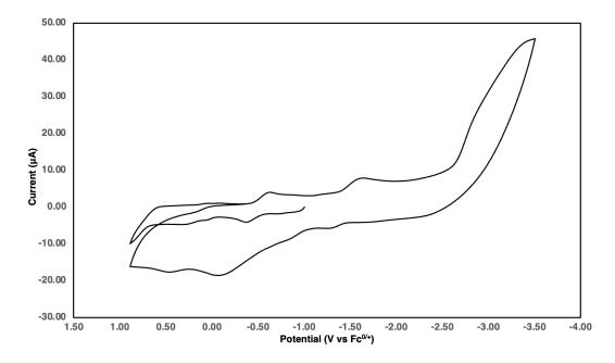
Figure S16. Cyclic Voltammogram of 2.4 mM of **1** in 0.1M KPF<sub>6</sub> electrolyte in a 1:4
