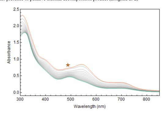
Figure S5. UV-vis of **1** from a 0.13 mM solution in toluene at room temperature heated for 60 °C for 3 hours (same decomposition occurs at RT at a slower rate). Orange marker indicates presence of putative thermal decomposition product (assigned as **2**)
