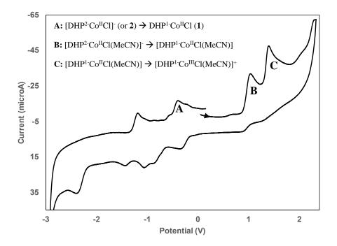
Figure S22. Cyclic Voltammogram of 1 mM of **1** in 0.1 M NBu<sub>4</sub>PF<sub>6</sub> acetonitrile (arrow placed at beginning of scan).
