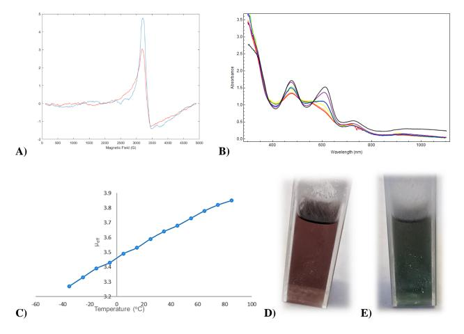
Figure 4. A) Integrated Variable Temperature EPR Spectra (16 K-22 K); B) 297 K to 173 K (black to red), individual scans at each temperature in 1 MeCN: 10 2-methyl THF, scan speed 1200 nm/min. C) Variable Temperature Evans Method in 1 CD<sub>3</sub>CN: 10 d<sub>8</sub>-toluene—358 K to 238 K.
