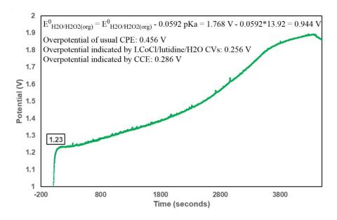
Figure S35. Bulk electrolysis at fixed 5.2 mA current in the presence of 1 mM 1, 320\*2 equiv.
