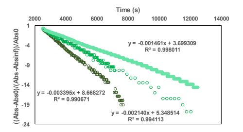
Figure S16. Linear fits in the second order fits of the data shown above (as well as check for reproducibility in the reaction of **1-OH** at 0.094 mM, 0.043 mM, and 0.078 mM) with MeCN at 2  $^{\circ}$ C in diethyl ether. k<sub>obs</sub> = 0.0023(8).
