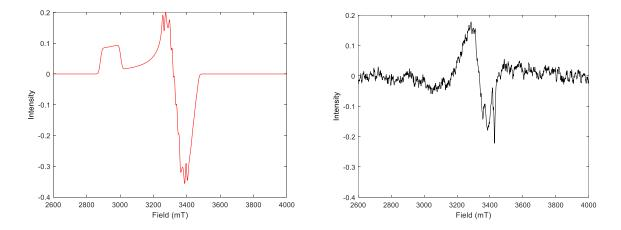
Figure S21. Small Window perpendicular-mode EPR spectrum (right) and simulated spectrum (left) of a 15 mM solution of [<sup>*t*Bu, Tol</sup>DHP]CoOH in toluene at 25 K. Conditions: MW frequency, 9.63 GHz; MW power, 2.0 mW.
