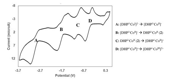
Figure S24. Cyclic Voltammogram of 1 mM of 2 in 0.1 M NBu<sub>4</sub>PF<sub>6</sub> tetrahydrofuran.
