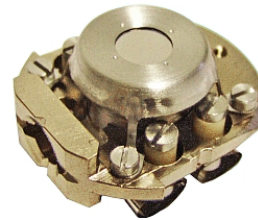
Figure A.5: Sample cartridge for the ELMITEC PEEM system. The sample is mounted by screwing a cap with a circle opening from the top. A thermocouple wire is in physical contact with the back of the sample, allowing accurate temperature reading.
