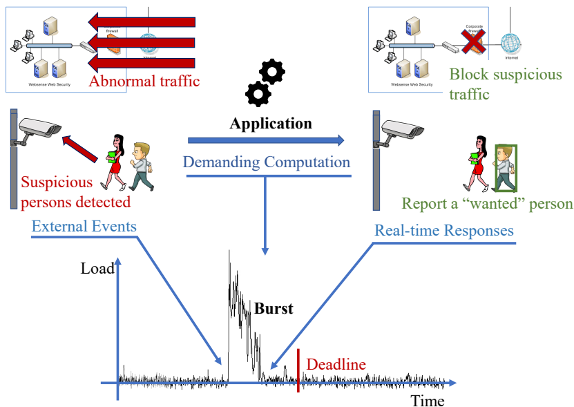
Figure 1.3: Bursty, real-time application examples: External events, such as cyberattacks and pedestrian appearance, trigger applications to start demanding computation with a strict deadline. The application consumes significantly more resources than usual (i.e., burst) to respond (e.g., block suspicious traffic and detect identities) in time.
