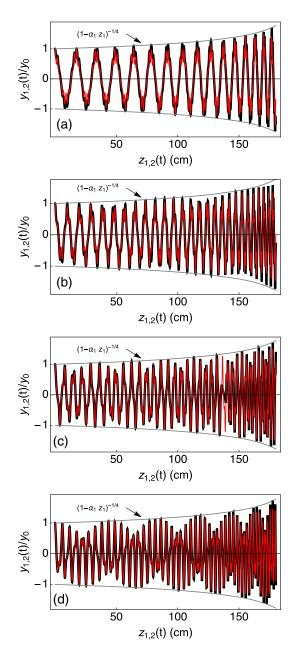
FIG. 6. Trajectories  $y_{1,2}(t)$  of a first particle (black) and second particle (red) versus particle longitudinal coordinate  $z_{1,2}(t)$  for (a)  $\Phi_1 = 0.227\pi$ , w(s)/K = 0.12, f(s) = 0.484; (b)  $\Phi_1 = 0.389\pi$ , w(s)/K = 0.13, f(s) = 0.344; (c)  $\Phi_1 = 0.525\pi$ , w(s)/K = 0.08, f(s) = 0.164; (d)  $\Phi_1 = 0.689\pi$ , w(s)/K = 0.056, f(s) = 0.09.
