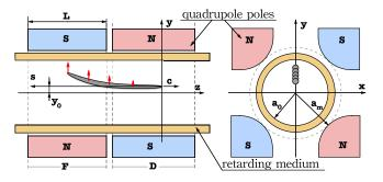
FIG. 1. A schematic diagram of the CWA embedded in the FD channel and the electron bunch propagating from the left to right.
