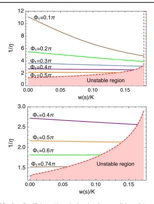
FIG. 5. Coefficient  $1/\eta$  calculated using condition (34) and formula (31) for different values of phase advance  $\Phi_1$  of the first particle (35) as a function of normalized wakefield; lower panel: zoom of coefficient  $1/\eta$  to higher phase advances.
