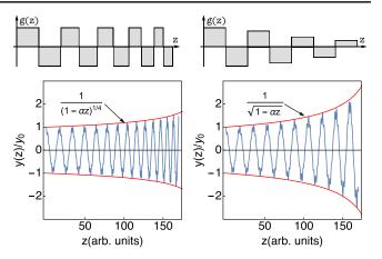
FIG. 2. Solution of Eq. (1) for s = 0, loss parameter  $\alpha = 0.005$ and maximum  $\sqrt{K}L = 0.35\pi$  (phase advance  $0.2266\pi$ ) for adaptive beam focusing using lens length variation  $L \propto \sqrt{1 - \alpha z}$ (left panel) and lens magnetic gradient variation  $g_0 \propto (1 - \alpha z)$ (right panel).
