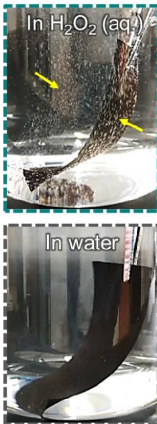
Fig. S17. Demonstration of bubble generation of M-MPN-M (arrows point to oxygen bubbles).
