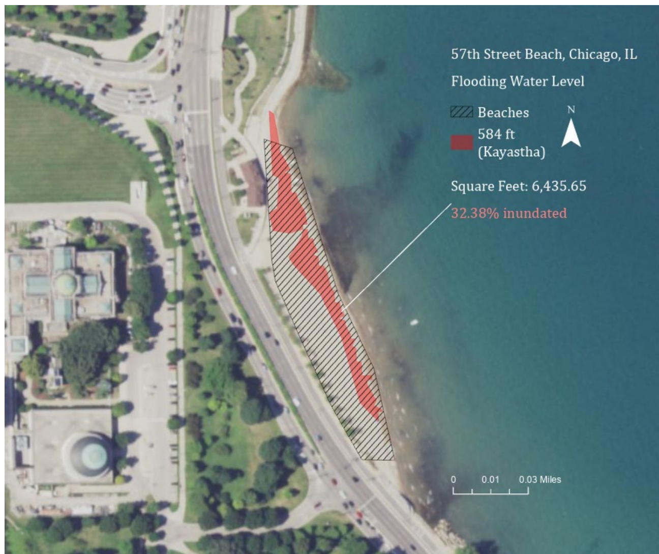
Image 2.2: Inundation model of 57 th Street Beach in Chicago, IL under the 584 ft. scenario.
