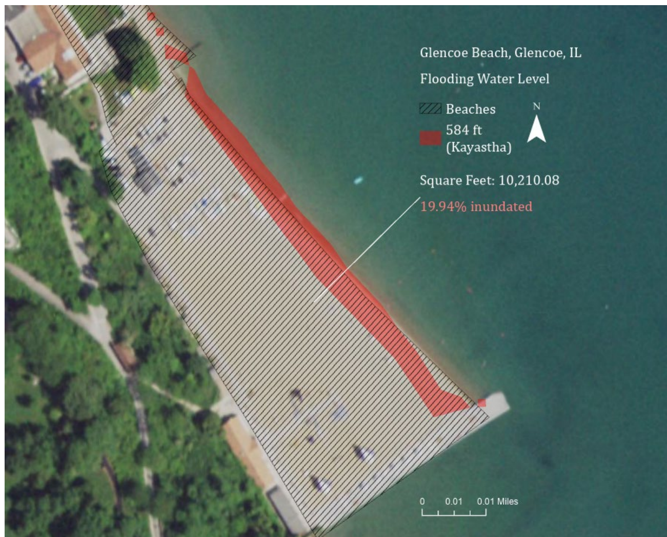
Image 2.1: Inundation model of Glencoe Beach in Glencoe, IL under the 584 ft. scenario.
