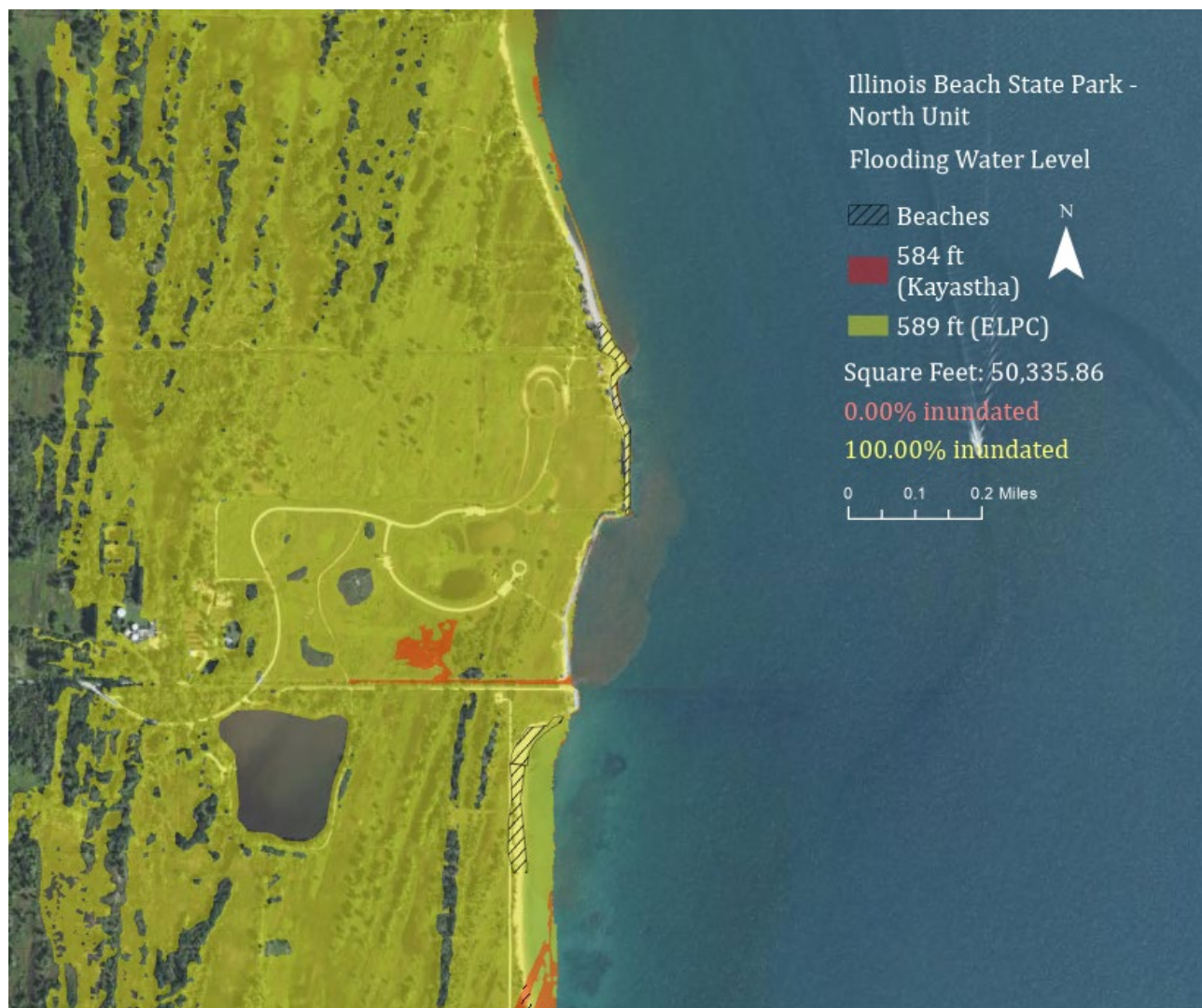
Image 5.2: Inundation model of the IBSP North Unit using predictions from both the 584 ft. and 589 ft. scenarios.
