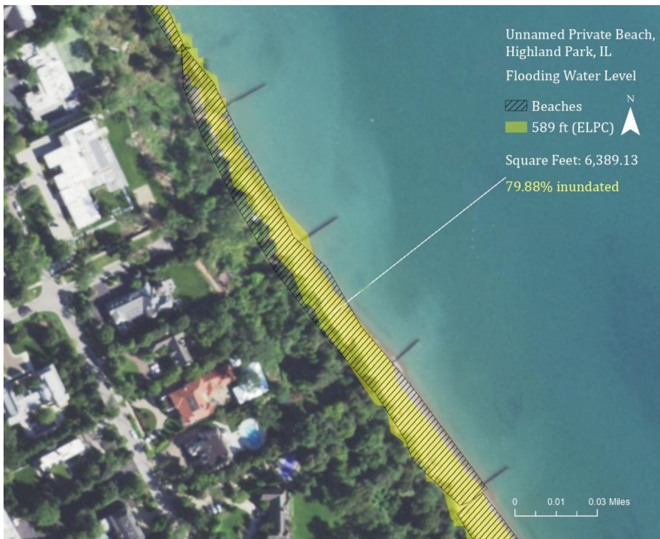
Image 1.1: Inundation model of a private beach in Highland Park, IL under the 589 ft. scenario.
