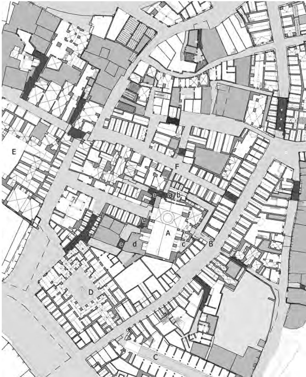
Fig. 9. Tripoli, ‘Aṭṭār Mosque–A. Ground plan: a–minaret; b–latrine; c–courtyard; d–room bordering to the southwest; e–enclosing passageways. B–Sūq al-Bāzirkān; C–Khān al-Miṣriyīn; D–Khān al-Khayyāṭīn; E–Khān al-Jāwīsh; F–Zuqāq al-Tarbī‘ah.
